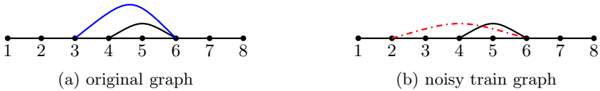
Fig. 1. Original graph before (Figure a) and after (Figure b) adding noise (dashed red edge) using the same link prediction algorithm (Adamic/Adar method). Adding noise edge (2, 6) in Figure (b) improves link prediction performance, as observed by the %23 and %250 increase in the values of link prediction quantitative criteria ( ROC and Average Precision , here). (Color figure online)
